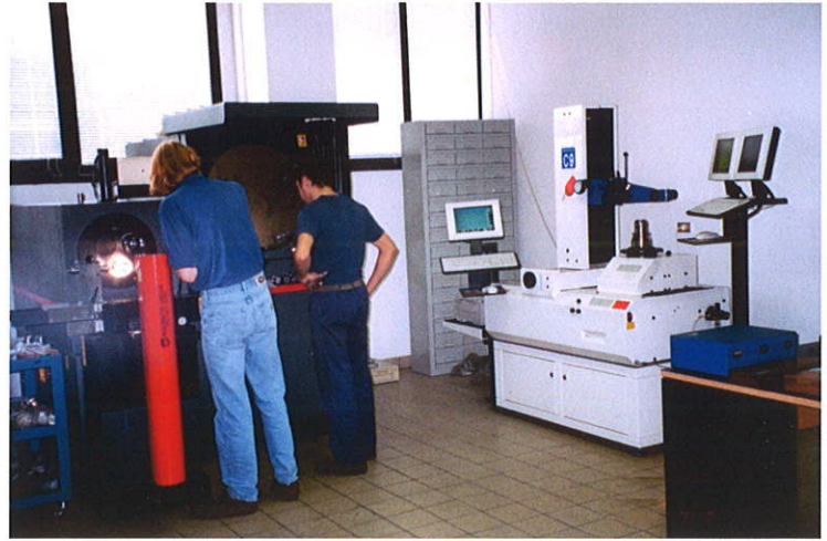
Laser measurement machine without contact with work piece
